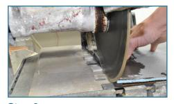
**Step 6** Place downward pressure on the top layer of cement board, turn the saw on and slowly proceed with cutting. The downward pressure should be sufficient to compress the weather-strip, preventing water from flowing under the board, and stabilize the mosaic tiles during cutting.
