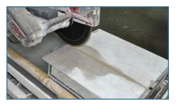
Step 1 Cover the saw tray with a piece of 1/4" cement board. This will provide a continuous surface that supports the sheet during cutting and prevents mosaic pieces from falling into the tray's cutting channel.
